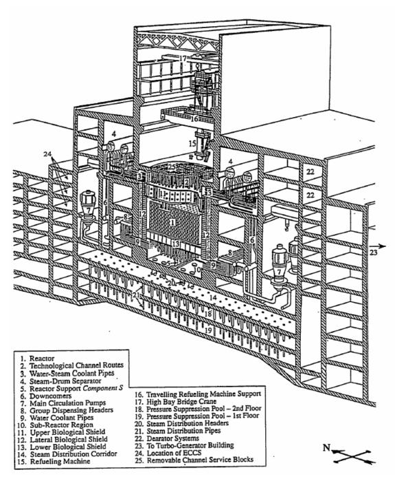
Figure 1: Intact Chernobyl Unit 4 Cross-Section<sup>6</sup>
