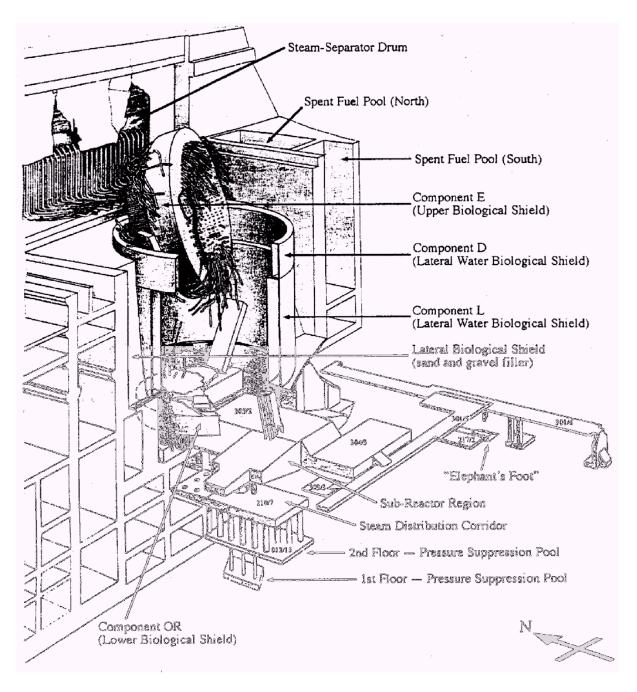
Figure 2: Post-Accident Chernobyl Unit 4 Cross-Section with LFCM Pathways<sup>3</sup>
