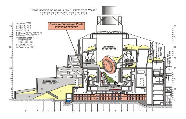
Figure 3: Chernobyl Unit 4 Shelter Cross-Section<sup>1</sup>
