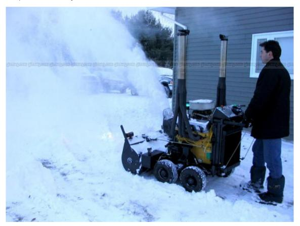
The first point to make is that this is not a V8 grafted on a traditional snow blower carriage but a purpose-built unit crafted around a motor of this magnitude. It functions very much like a traditional blower by way of operator input and feedback and offers effortless safe operation.
